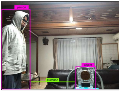
Fig. 14 Person-object distance measurement
